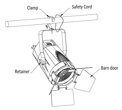
The unit was designed to make installation easy: The fixture's head can be rotated within 240° manually, before it rotates, two side retainers are loosened with care; after the head at a desired angle, tighten two side retainers..
