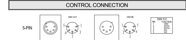
Connection between the controller and a projector and between one projector and another must be made with a 2 core-screened cable, with each core having at least a 0.5mm diameter. Please use the projector's cannon 5- pin signal input and output cables as connection. The 5-pin signal connections are connected as shown in the figure above.
